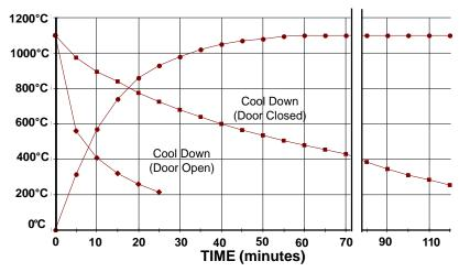
Test Conditions: Nominal line voltage, no load in the muffle only floor tray, full power applied to the muffle for the Heating Curve. The programmable rates are linear and fall <u>below</u> the heating curve and <u>above</u> the cooling curve (door closed) for some selections.
